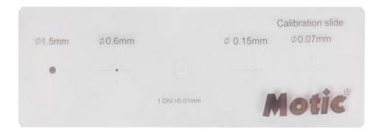
**1-** Once the dot is perfectly focused, and without it protruding from the field of view on the window, we will need to go to the "advanced settings" menu and select the option "calibration".
